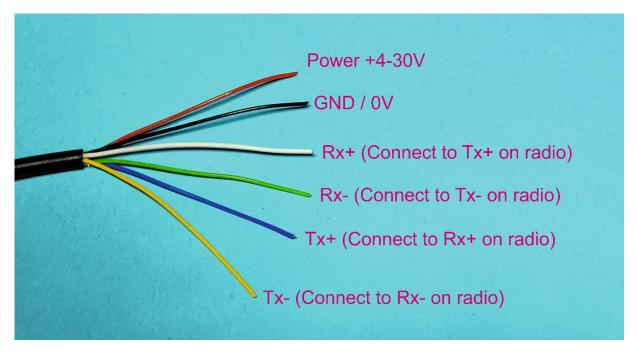
Tx from radio shall be connected to Rx on Aviation Companion 422 and vice versa.
