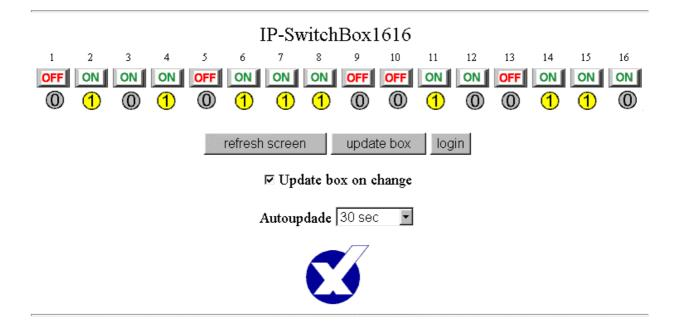
When you click at the ON or OFF button a request for this is sent to the box. Then the button turns gray until the box has confirmed the change. When the confirmation arrives the button indicates current setting again.
