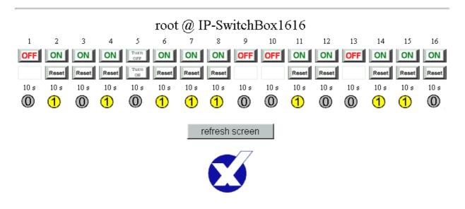
On output 5 a reset is started. The Reset can be cancelled by clicking "Turn ON" or "Turn OFF".
